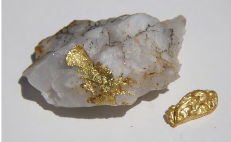
Lode gold in quartz and a nugget of placer gold panned from a riverbed.
