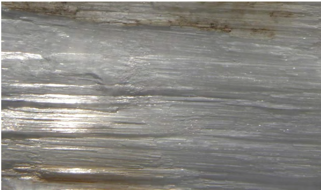
Ulexite often has closely packed crystal bundles running parallel to one another.
