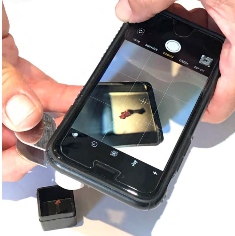
Don't have a microscope? Craft one from a cell phone camera and a loupe!
