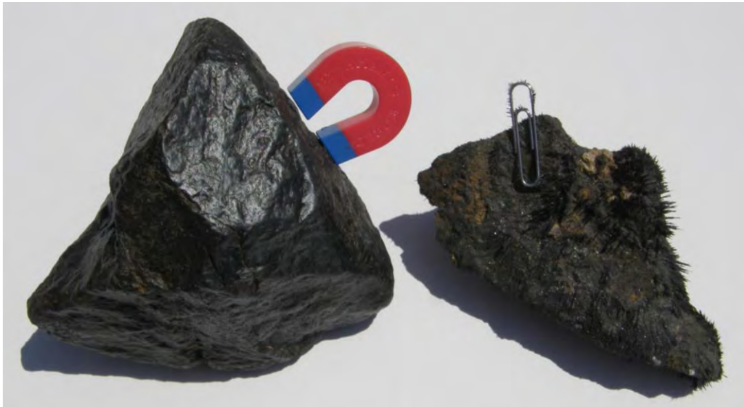
Magnetite (left) attracts a magnet while lodestone magnetite (right) is a magnet!
