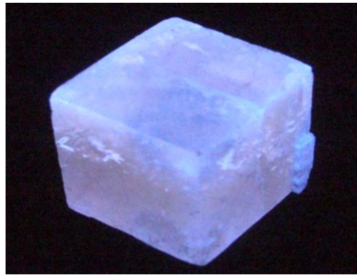
Calcite can exhibit a brief "afterglow" after exposure to a UV lamp.
